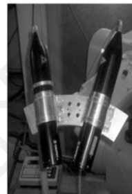
Fig. 2 View of the laser probes fixed on the robot arm and the three-dimensional laser probe system.
